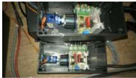
Figure 9. The Dimmer and Servo Motor In The Box
